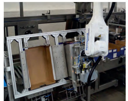
The robot moves products down into the box in controlled programmed movements so collision and stops are avoided.
